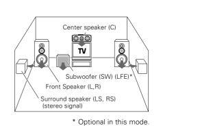
\* LFE = Low Frequency Effects. This channel delivers separate non-directional bass signals to the subwoofer for more dynamic deep bass sound effects. Dolby Digital is the only Dolby method to have an LFE channel.
